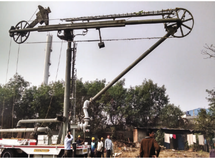
Client : Coromandel International Ltd, Kakinada Trailer Mounted Marine Loading Arm along with Jumper Assembly for Liquid Ammonia (Size :8" x50")
